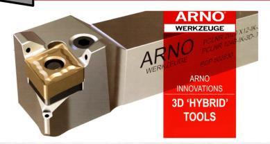
How do you improve turning performance? Get coolant to the cut zones through 3 ports with one under the insert flank. Eliminate the top clamp that is prone to damage and just gets in the way. Then 3D print the tool for smooth high volume channels without restrictive cross drilling. More coolant and no special hardware, that's the 3D Hybrid indexable turning tool from Arno.
