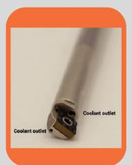
The challenge to build a vibration damped turning tool small enough for this application has been solved by MAO! They have designed it with through-coolant capability because it's critically important to excavate chips out of small holes.
