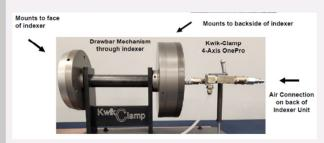
The OnePro systems are the one product for mounting any workholding. NO NEED for any housing, risers, extra mounts lifters, etc. to work.
