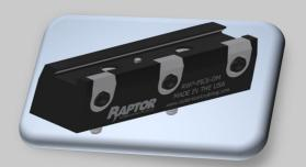
Raptor Picatinny Fixtures are made to hold your part on four and five-axis CNC machines. The fixtures provide rigid clamping while exposing five faces of the workpiece – Most features can be completed in a single operation. Our unique Raptor Picatinny spring-loaded clamps are designed to fit the industry standard to hold the rails. You prepare a picatinny rail on your first operation, and this fixture will hold your final operation. Easy, strong and efficient.
