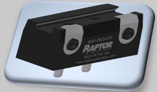
Raptor Picatinny Fixtures are made to hold your part on four and five-axis CNC machines. The fixtures provide rigid clamping while exposing five faces of the workpiece – Most features can be completed in a single operation. Our unique Raptor Picatinny spring-loaded clamps are designed to fit the industry standard to hold the rails. You prepare a picatinny rail on your first operation, and this fixture will hold your final operation. Easy, strong and efficient.
